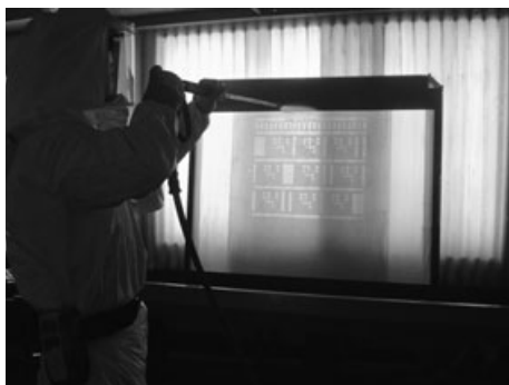
15.13 Technician cleaning plastic sheets with ink containing SWCNTs (courtesy Mary Schubauer-Berigan and Matt Dahm, NIOSH).
