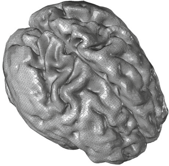
Fig. 7.13 Hex-mesh generated on human brain
