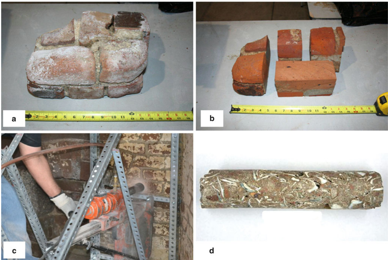
Fig. 51.5 (a) Block specimen from the remains of the fort; (b) block specimen segmented into smaller samples for testing; (c) coring of the wall in progress; (d) an intact core sample of tabby concrete infill
