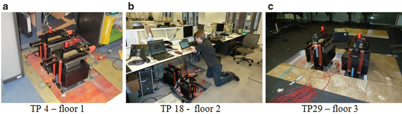
Fig. 5.4 Typical collocated sensor and actuator pairs at TPs 4, 18 and 29 in floors 1, 2 and 3 (a–c), respectively (note that the additional shaker here is used for uncontrolled and controlled FRF tests only)
