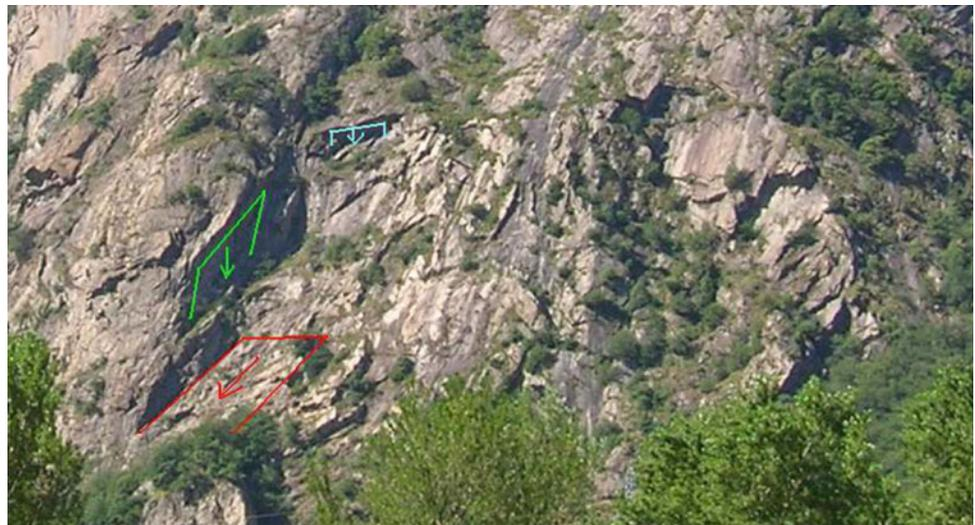
corresponding orientation that is derived computing the best fitting surface of the selected points. The high quality of solid images has allowed to interpret rock mass quality according to the GSI index also for impervious areas.
