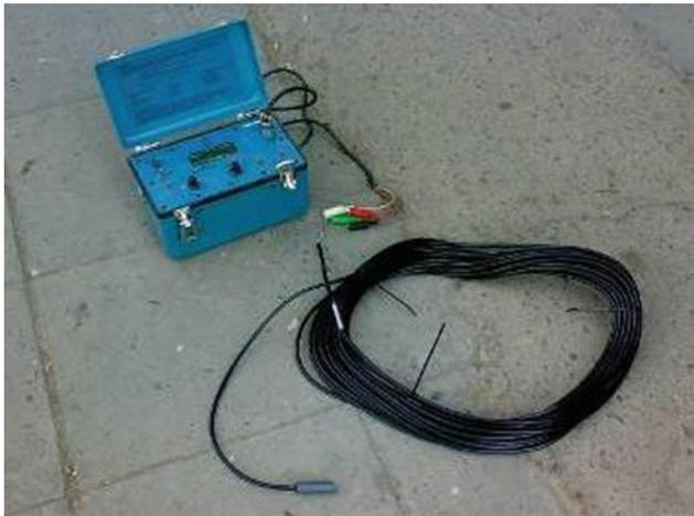
**Fig. 49.2** Electrical thermometer tool
