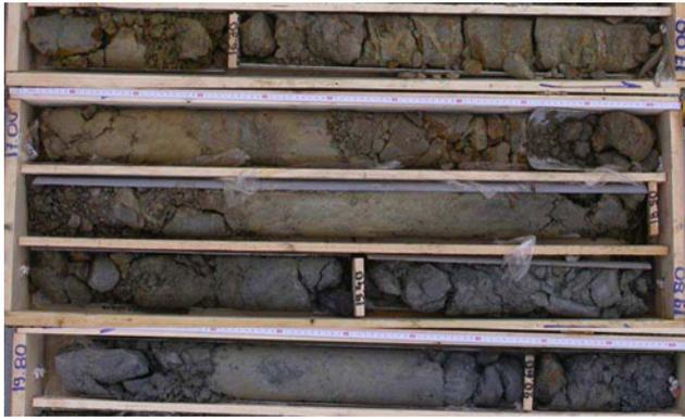
**Fig. 151.1** Typical transition from the upper to the lower Athens Schist. The transition is marked by the presence of a shear zone between 17.9–19.3 m
