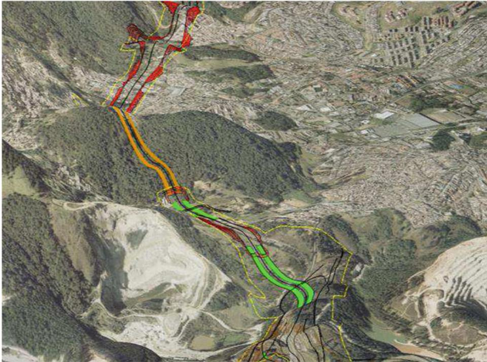
**Fig. 195.1** Highway segment. Satellite image overlapped on the DTM. *Green* bridge or overpass; *orange* tunnel; *red* cut and fill; *yellow* right of way
