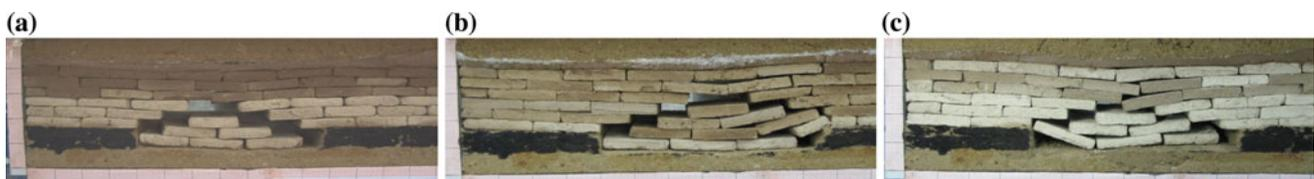
**Fig. 146.1** Affect of formation combination to the deformation of dual structure. **a** Soft-hard combination. **b** Soft-soft combination. **c** Hard-hard combination
