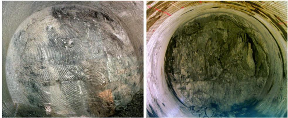
performance in areas of face spalling can be improved or reduced depending on the severity of spalling (Kaiser 2005), irrespective of the impact of spalling at the walls. Consideration must, therefore, be taken for spalling at the face, even if spalling at the walls is not anticipated. This paper shows how stress and geomechanical characteristics affect excavation and presents a characterisation scheme to identify conditions where advance rates can be impacted by spalling at the tunnel face.
