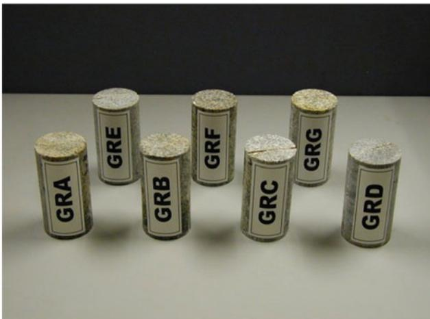
**Fig. 160.1** Core specimens used for the measurements of roughness
