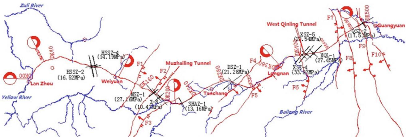
**Fig. 3.2** Geological stresses measured along the railway line from China Railway First Survey and Design Inst
