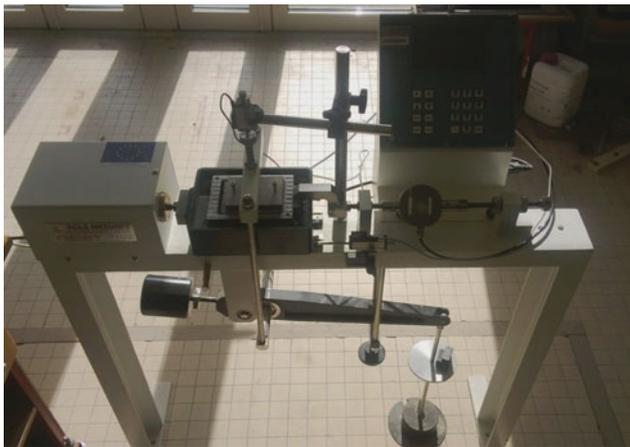
**Fig. 145.4** Experimental shear test equipment
