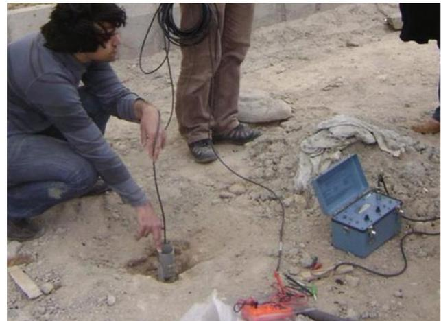
**Fig. 49.3** Natural ground temperature measurements
