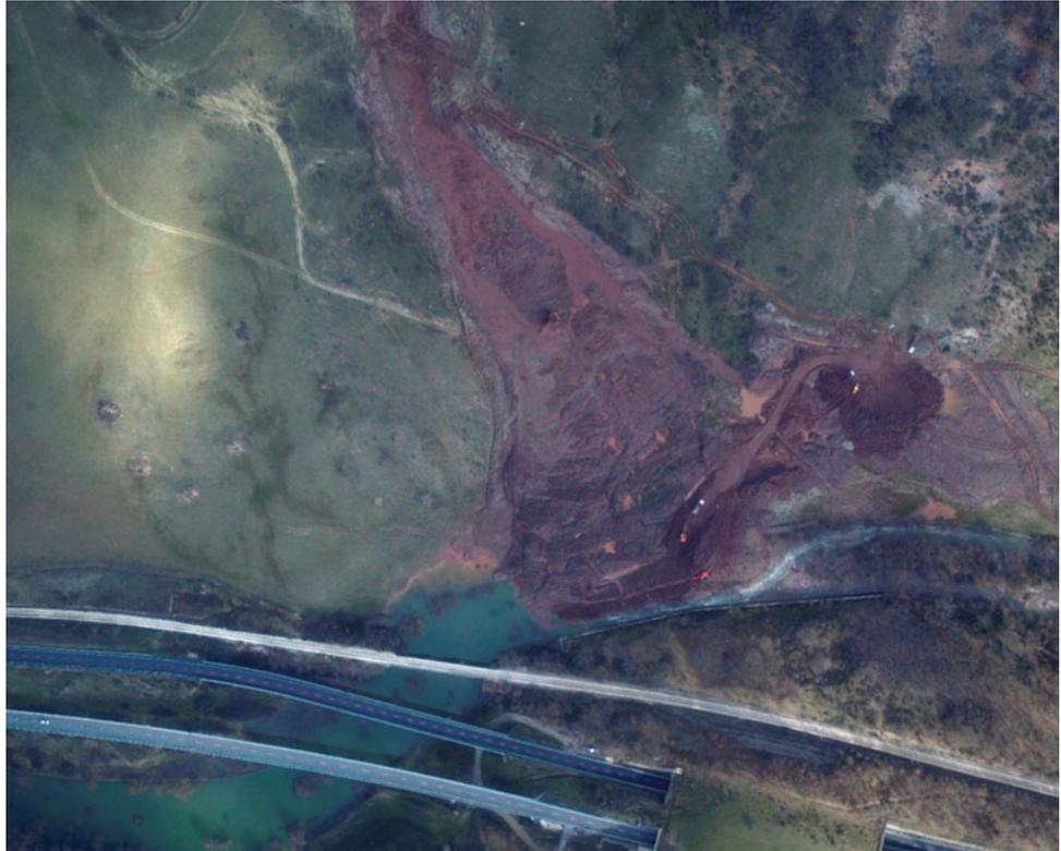
**Fig. 135.2** Basento River occluded by landslide debris and parts of existing retaining wall
