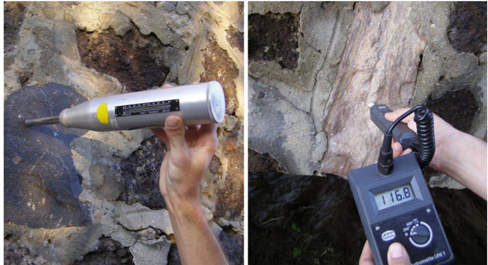
The condition of the mortar, the potential damages (missing blocks, cracks) have to be observed on site as well. If sampling is possible then core samples from the backfill and from the blocks should be taken for laboratory analysis.
