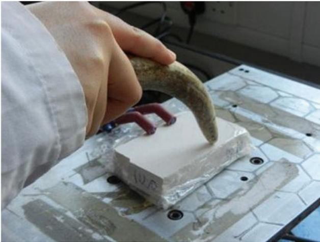
**Fig. 53.5** Forming a groove on a sample of chalk clamped to a force plate
