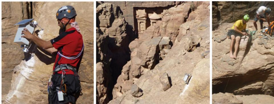
inclination of the blocks and meteorological parameters are the main data collected by the system.
