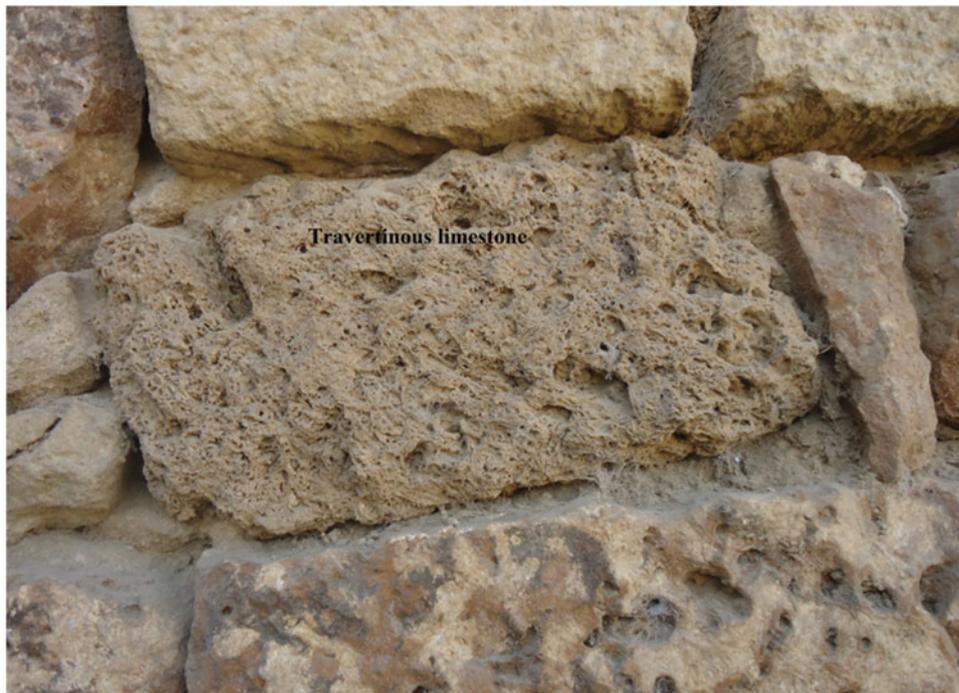
**Fig. 27.2** Travertinous highly porous limestone
