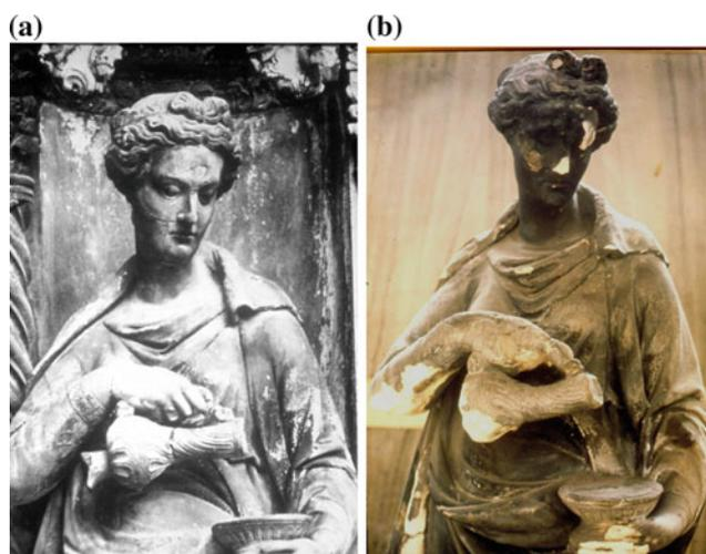
**Fig. 3.1** a, b. Temperance statue, Carrara marble. In 1900 (*left*) the state of conservation was rather good, in 1976 (*right*) some missing parts are visible due to marble dechoesion after heavy atmospheric pollution exposure
