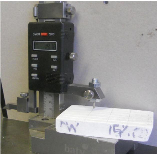
**Fig. 53.6** Measuring depth of surface markings
