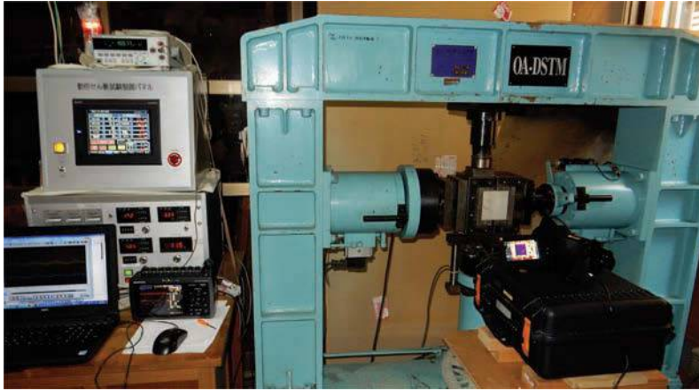
Figure 2.5 Multi-purpose dynamic shear-testing machine with a capability to perform creep tests on rocks, discontinuities and interfaces at the University of the Ryukyus.
