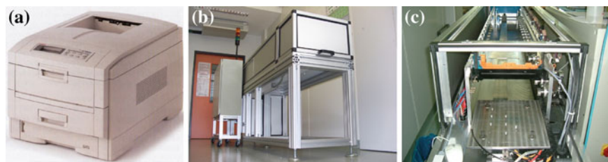
Fig. 1.5 Prototype of the peptide laser printer. a OKI C7400 laser printer; b Peptide laser printer (closed); c Printing track without cartridges
