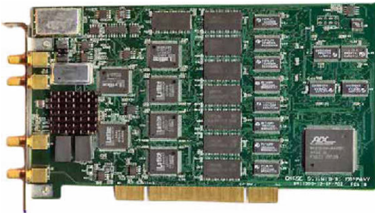
Fig. 2.11 The PCB of PCI based Arbitrary Waveform Generator [25]
