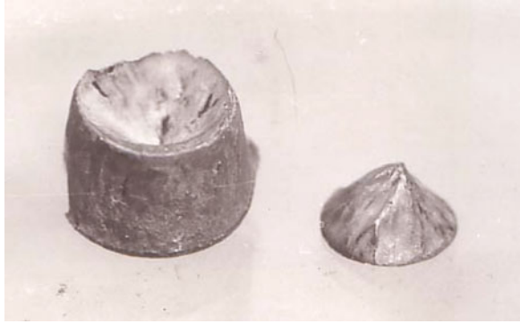
Fig. 8.4 The typical plug and cone after complete perforation of 60 mm thick aluminium alloy target. Melting cone surfaces are formed by intensive plastic shear deformations. The projectile velocity V_0 = 660 m/s. Plug and cone heights are 15 and 8 mm, respectively [14]
