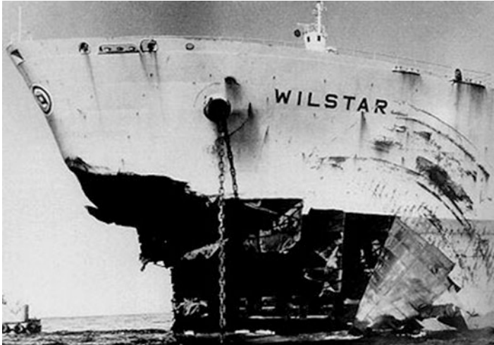
Fig. 6.18 The damage received by Norwegian tanker Wilstar in 1974. The combination of ship motion and a steep incoming wave can cause extreme local structural damage. Internet. https://www.flickr.com/photos/40269779@N08/3928691965/
