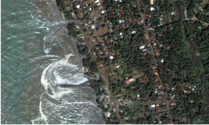
Fig. 5.1 Evolution of the 2004 Indian Ocean tsunami near the coast of Sri Lanka: the form changes from the wall of water ( low part ), through the breaker to the localized jet ( upper part ) [6]
