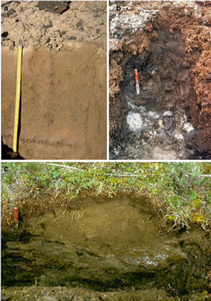
Fig. 8.3 Representative soils in the Canadian Arctic: (a) Static cryosols, (b) Organic cryosols, and (c) Turbic cryosols. Note the ice ( white areas ) in the lower part of soil profiles b and c (Tarnocai and Bockheim 2011)
