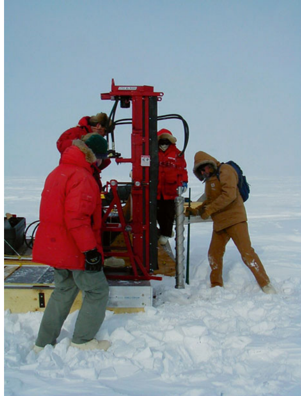
Fig. 3.6 Gasoline-powered drill rig with a SIPRE core barrel for sampling permafrost in arctic Alaska. The drill rig is carried on a sledge that is pulled by a snow machine (Photo by J. Kimble)
