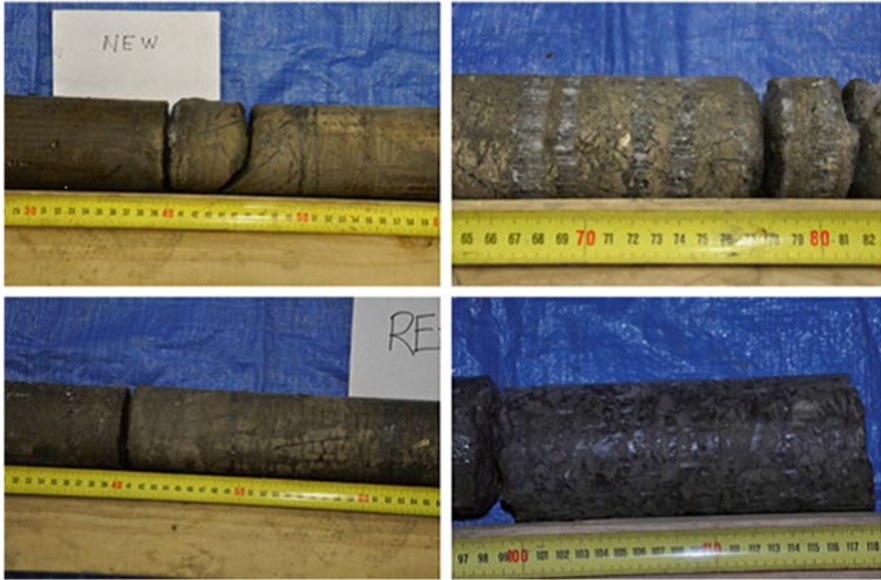
Fig. 2.8 Forms of excess ice in cores from drained thaw-lake basins in arctic Alaska, including vein ice ( upper left ), lens ice ( upper right ), reticular ice ( lower left ), and ataxatic ice ( lower right ) (Bockheim and Hinkel 2012)
