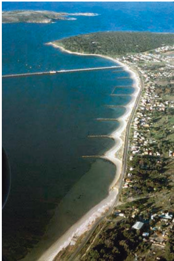
Fig. 3.4 Groynes containing sandy beach compartments on the south coast of Botany Bay, New South Wales. © Geostudies
