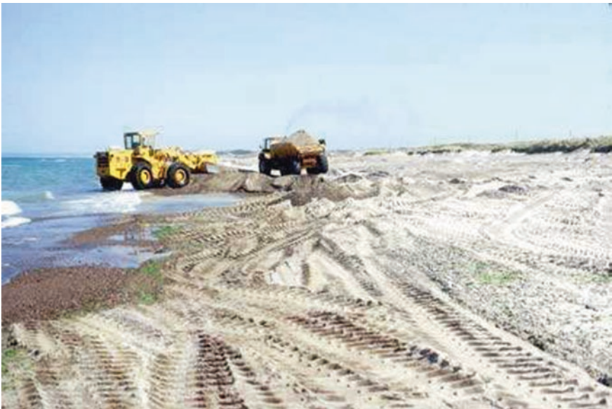
Fig. 2.17 Extraction of sand and gravel from the beach at Klim in Denmark. © Geostudies
