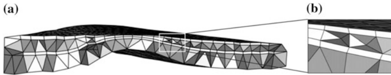
Fig. 4.14 a Conformal hybrid grid consisting of tetrahedra, triangular prisms and pyramids; with b details showing a perfect fitting with the horizons (from Pellerin et al. 2012)
