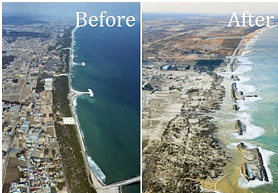
Fig. 16.7 Aerial photos of the Yamamoto Coast before ( left ) and after the tsunami ( right ) taken by MLIT (March 27, 2010) and Kyodo News (March 9, 2011)
