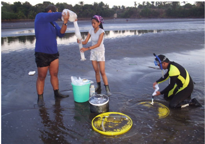
Fig. 2.10 Measurement and sampling SGD using seepage meters during the low tide period
