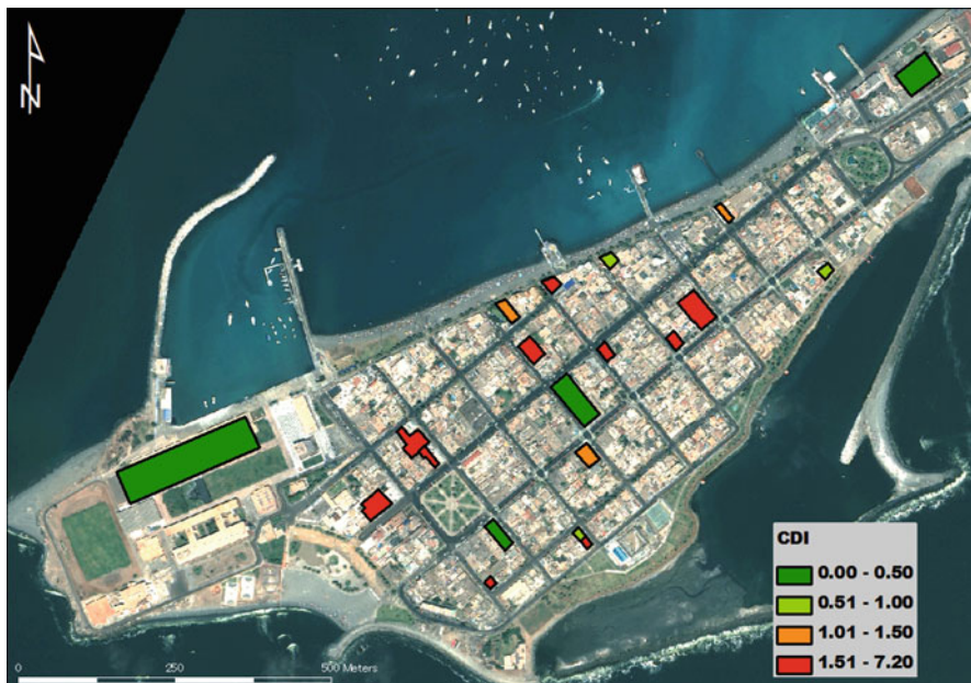
Fig. 19.10 Capacity-Demand mapping of TEBs. CDI > 1.0 (over demand) – CDI < 1.0 (under demand) (H&V case)
