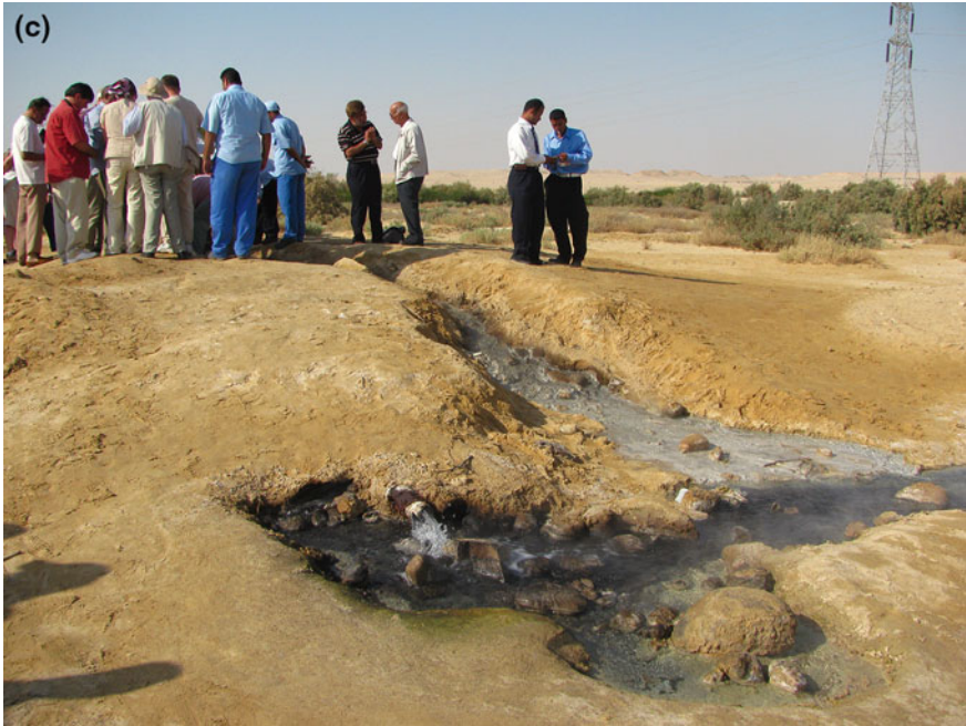
Photo 10 a, b, c Ras Badrun oil field, Sinai Peninsula: old oil-well with artesian flow of thermal water. Outflow temperature measured by Dr. Balderer was 64.9 °C (photo 10b)
