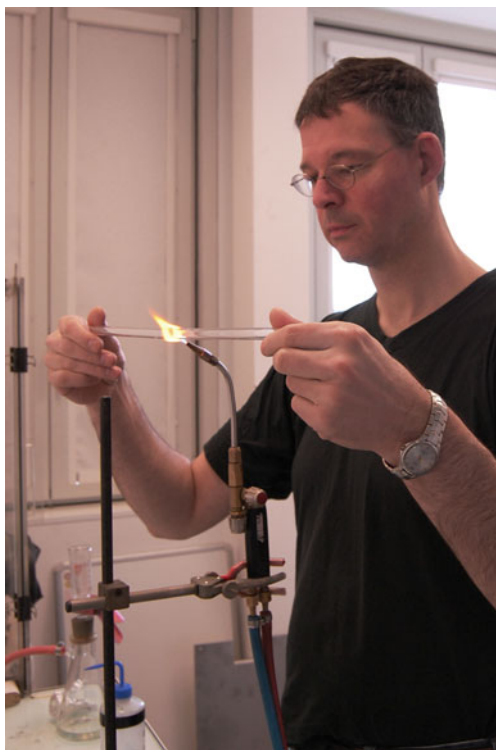
Fig. 4.1 Photograph showing the writer while melting a piece of glass tubing into two reaction tubes. Photograph taken by MHC Vlaanderen and used with permission
