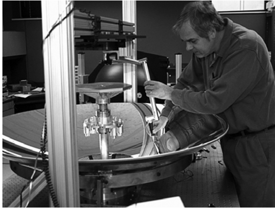
Fig. 5.9 Measurement of the primary mirror to identify the optical axis
