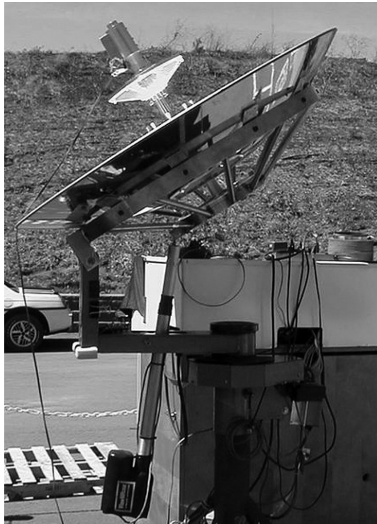
Fig. 5.10 Fully assembled prototype HSL concentrator and tracker
