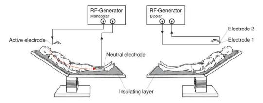
Fig. 6.2. Monopolar (i.e., Somnus) and bipolar (i.e., Celon) systems for interstitial radiofrequency surgery
