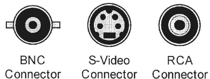
Figure 9-3: Standard Video Connectors
