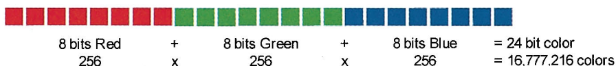
Figure 8-5: 24-bit color. This is the most popular color encoding scheme used for digital images and allows for more colors than can be discerned by the human eye.
