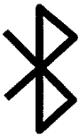
Figure 2-8: Bluetooth icon. Since Bluetooth is a wireless protocol, if a port is labeled with the Bluetooth icon, that connection is for an external antenna.
