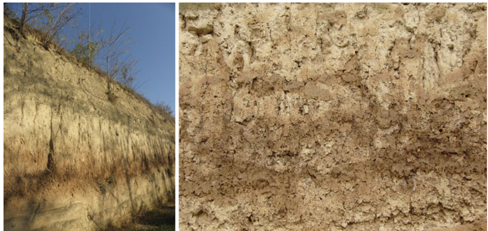
Photo 4.2 Typical calcareous loess with paleosol ( left ); close-up of the paleosol ( right ), eastern Pannonian subregion, city of Ilok
