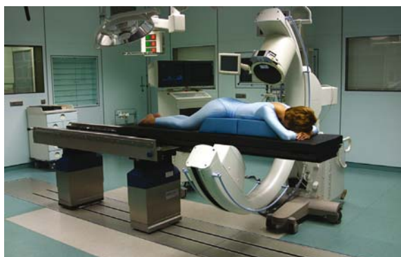
■ Fig. 6.26. Special table top for sliding gantry or C-arm
