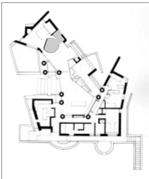
FIG 4. Second Solution: bathroom as an oval (shaded area at upper left)
