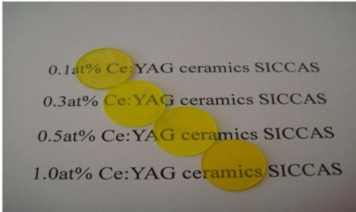
**Fig. 16.1** Photograph of  $\text{Ce}^{3+}$ -doped YAG transparent ceramics with different doping concentrations: 0.1 at. %, 0.3 at. %, 0.5 at. %, and 1.0 at. %.(double face polished,  $\varnothing 14 \text{ mm} \times 1.0 \text{ mm}$ ). Yellow color characterizes  $\text{Ce}^{3+}$  ions
