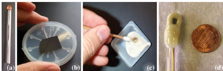
**Fig. 3.2** Connecting an electrode with Cu wire. Bare Cu wire is inserted into a glass tube and coiled at the end to increase surface area (a). The back side of the sample (b) is connected to the Cu coil using silver paint, followed by the addition of HYSOL 9462 epoxy (c) to encase the entire assembly. The finished product is shown in (d)
