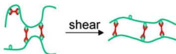
Fig. 15 Representation of the mechanism of shear thickening in pincer cross-linked PVP networks. Reproduced from [54] with permission from Copyright © 2010 American Chemical Society
