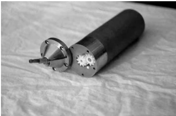
FIGURE 3.33 The PTFE drive gear of a gear-drive pump (center) meshes with a second PTFE gear to displace water (which enters the pump under hydrostatic pressure) through the pump chamber into the discharge tubing to the surface.
