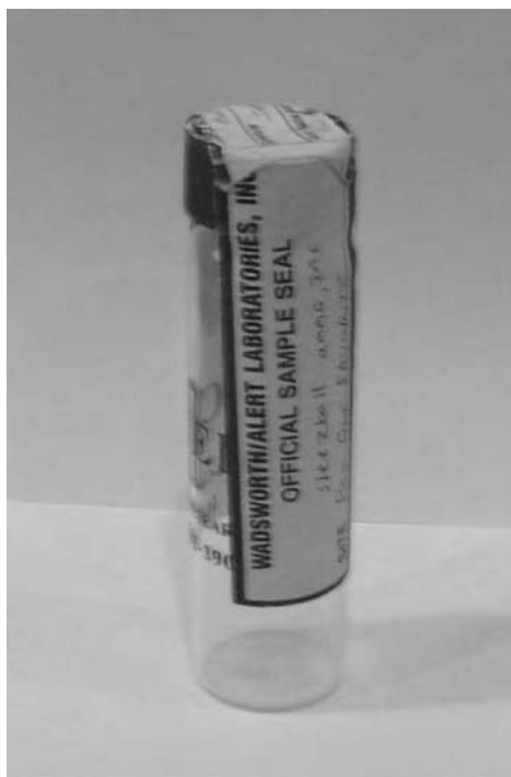
FIGURE 6.7 If the sample seal on a VOC vial covers the septum, the constituents of the adhesive from the seal may be detected in the analysis as the needle from the analytical instrument penetrates the septum to collect the sample.
