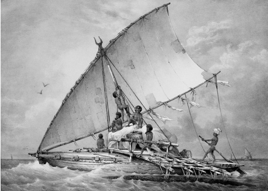
Fig. 2.5 A single hulled craft with an outrigger such as this Camakau from Fiji was one of many designs used throughout the Pacific islands as voyaging canoes. The framed sail is anchored to the forward part of the canoe and is supported by a central mast. Construction of the considerably larger drua required the replacement of the outrigger with a second hull ( Wikipedia.org )
