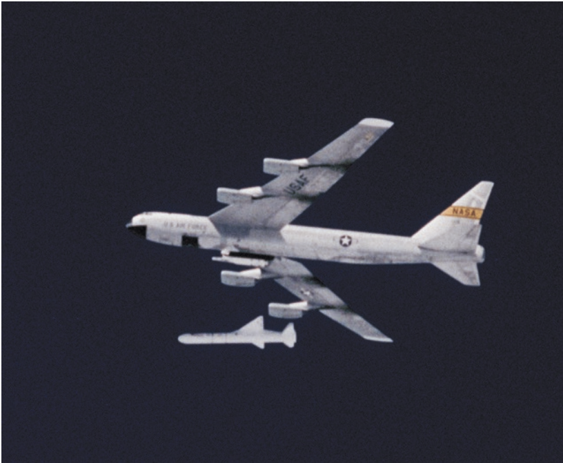
Fig. 9.5 A Pegasus booster seconds after being released from its B-52 carrier aircraft. (Courtesy of Orbital ATK Corporation.)
