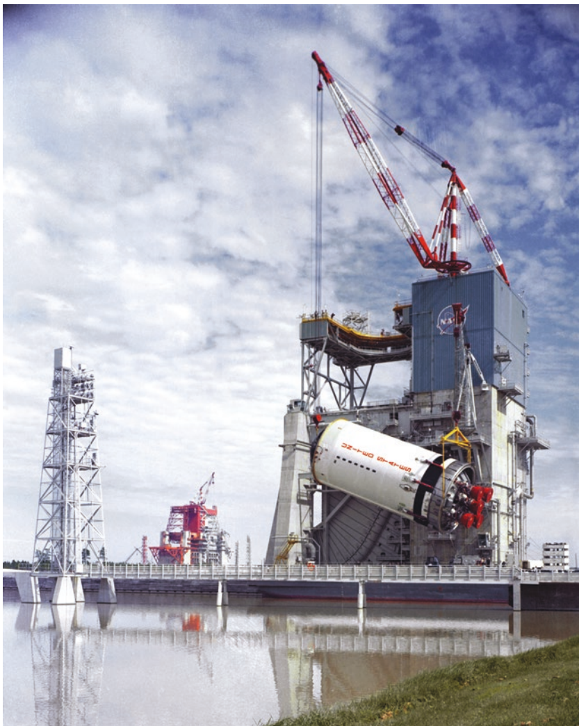
Fig. 1.1 Early spaceflight required advances in propulsion, computer technology, and orbital rendezvous. Here the S-II stage of the Saturn V rocket is hoisted onto the A-2 test stand in 1967 at the Mississippi Test Facility, now the Stennis Space Center. This was the second stage of the 364 foot tall Moon rocket. The second stage was powered by five J-2 engines. (NASA, image number 67-701-C, public domain) (Available at https://www.flickr.com/photos/nasacommons/9457467017/in/album-72157650356082218/ )
