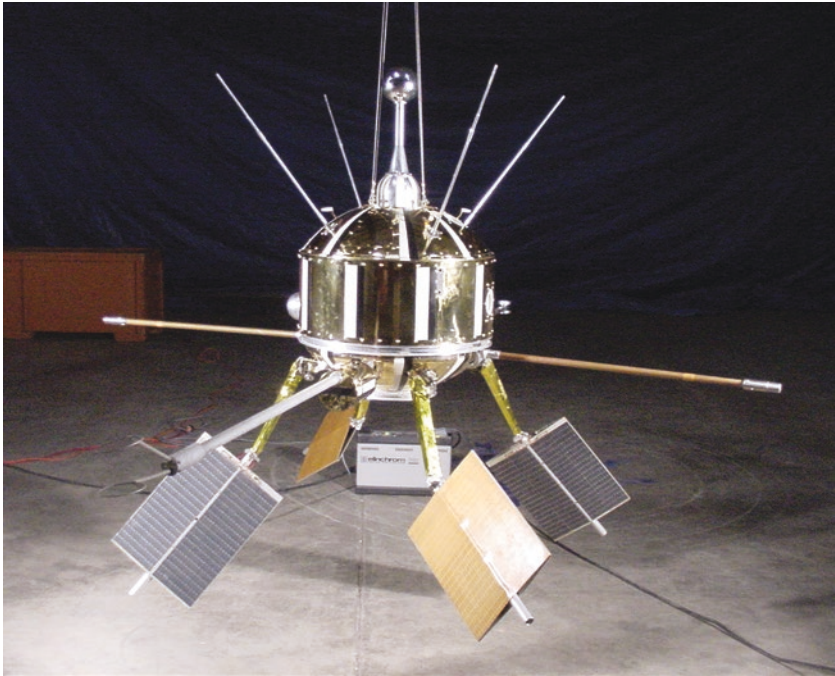
Fig. 2.2 A replica of Ariel 1, the world's first internationally conceived and executed satellite. The spacecraft carried six British experiments designed to study the ionosphere and its relationship to solar radiation, including cosmic ray, solar emission, and ionospheric experiments. The spacecraft chassis was built by the NASA Goddard Space Flight Center and launched on a Delta 9 launcher on April 26, 1962. (National Air and Space Museum, number A19751410000. Courtesy of NASM, Smithsonian Institution)
