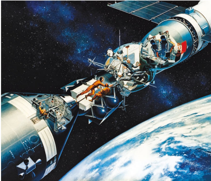
Fig. 8.3 This April 1975 NASA artwork by Davis Meltzer depicts a cutaway view of the international spacecraft created by the Apollo–Soyuz Test Project in July of that year. On the left, two American astronauts leave their crew mate in the Apollo command module to enter the docking adapter and meet their two Soviet cosmonaut counterparts in the Soyuz. NASA considered a follow-on mission that would have entailed joint US/Soviet operations aboard a successor to the Skylab Orbital Workshop. (NASA, image number S75-27290, public domain (Available at https://images.nasa.gov/#/details-S75-27290.html ))
