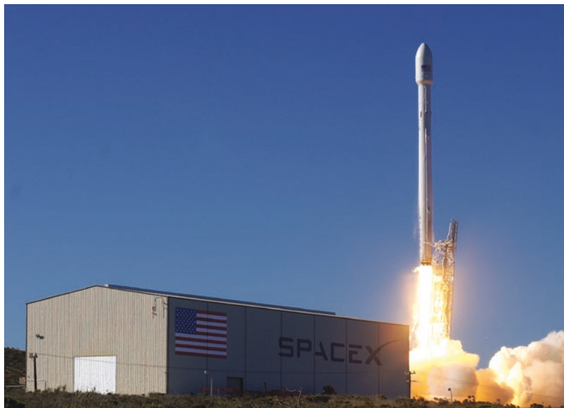
Fig. 13.1 Falcon 9 is a two-stage medium-lift range launch system. Created by SpaceX, Falcon 9 was intended to carry payloads to low-Earth and geosynchronous orbit. For its second launch In December 2010, the first Space X Dragon spacecraft was carried atop the launch system. (SpaceX, public domain.) (Available at http://www.spacex.com/news/2013/10/14/upgraded-falcon-9-mission-overview )
