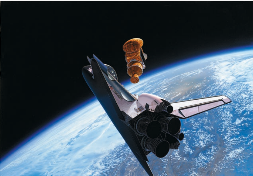
Fig. 9.3 An artist's concept of a transfer orbit stage and attached communication satellite being launched from the space shuttle. (Courtesy of Orbital ATK Corporation.)
