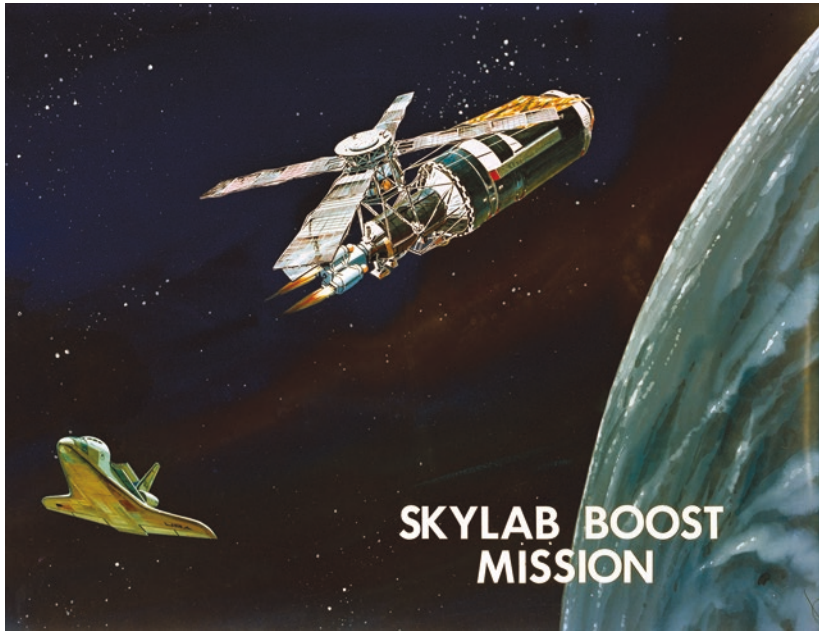
Fig. 8.4 This 1978 artist's conception depicts the Teleoperator Retrieval System being used to boost Skylab into a higher orbit, following the systems release from the space shuttle's cargo bay, on the left. The reboost mission was scheduled for 1979, but was never flown. (NASA, image number S78-23630, public domain (Available at https://images.nasa.gov/#/details-s78-23630.html ))
