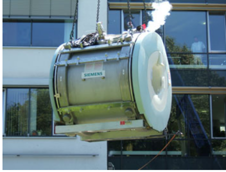
Figure 1.1: This MR scanner (MAGNETOM Trio, A Tim System 3T, Siemens Healthcare, Erlangen, Germany) was equipped with a PatLoc insert coil while this thesis was conducted. The scanner is shown during delivery to the site of installation. Visible from outside is the vacuum chamber that contains the main magnet, the largest component of the scanner.
