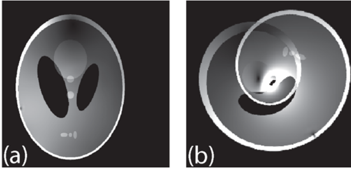
Figure 5.6: Deformed coil image with quadrupolar encoding. (a) Original magnetization weighted with the sensitivity of an RF-surface coil element. (b) Corresponding deformed image. The nonlinearities of the SEMs cause intensity modulation (increase toward the center) and severe image distortions. The non-bijectiveness of the encoding function is responsible for the fold-over. The effects - increasing information at the periphery and fold-over along the azimuthal direction correspond to the transformation induced by the encoding function, presented in Fig. 5.5.
