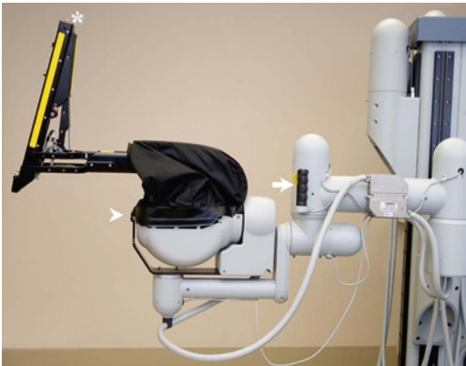
Fig. 2.12 Photograph of the da Vinci® standard instrument arm showing the port clutch joystick button ( arrow ), port clutch button ( arrowhead ) and instrument clutch button ( asterisks ) used to position the arm for draping, docking and storage
