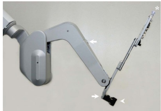
Fig. 2.14 Photograph of the da Vinci® S and HD instrument arm showing the port clutch buttons ( arrows ) and instrument clutch button with LED indicator ( asterisks ). Also seen is the trocar mount ( arrowhead )
