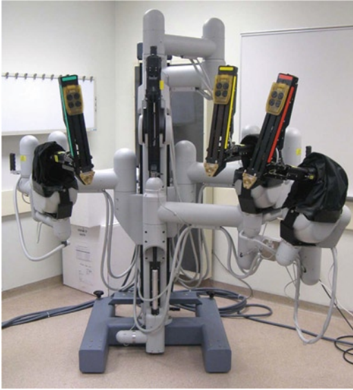
Fig. 2.11 Photograph of the da Vinci® standard patient cart with optional third instrument arm
