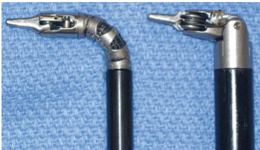
Fig. 2.20 Photograph of EndoWrist® needle drivers. On the left is a 5 mm needle driver with the “snake joint” compared to the 8 mm needle driver with an “angled joint”
