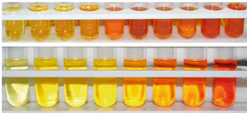
Fig. 1.10 Colloidal CdSe nanoparticles prepared at 150°C during 1, 5, 10, 15, 20, 25, 30, and 35 min of reaction times
