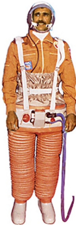
FIGURE 7.5 Lower Body Negative Pressure (LBNP) suit. One suspects that the only reason that the cosmonaut pictured is smiling is because his LBNP suit is not turned on. (Photo courtesy of NASA)
