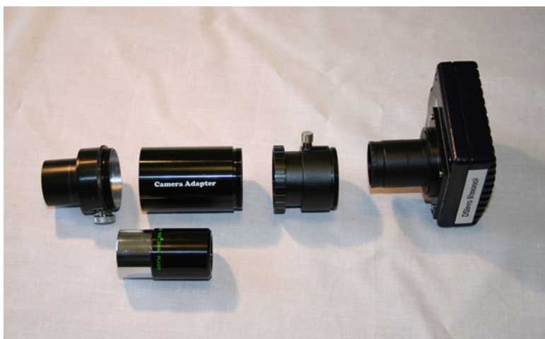
Fig. 5.9 Components for a transmission grating slit
