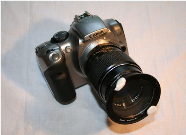
Fig. 5.13 Cokin Cosmos filter mounted on a 135 mm lens
