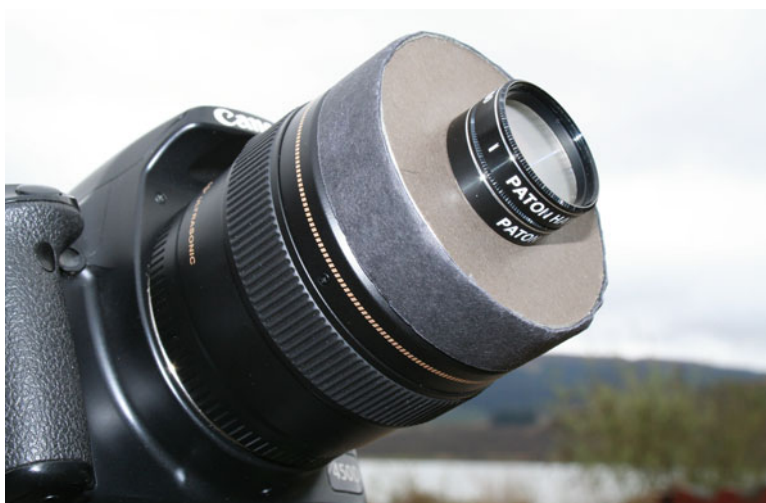
Fig. 2.12 A simple lens cap to hold the objective grating (J. Simpson)
