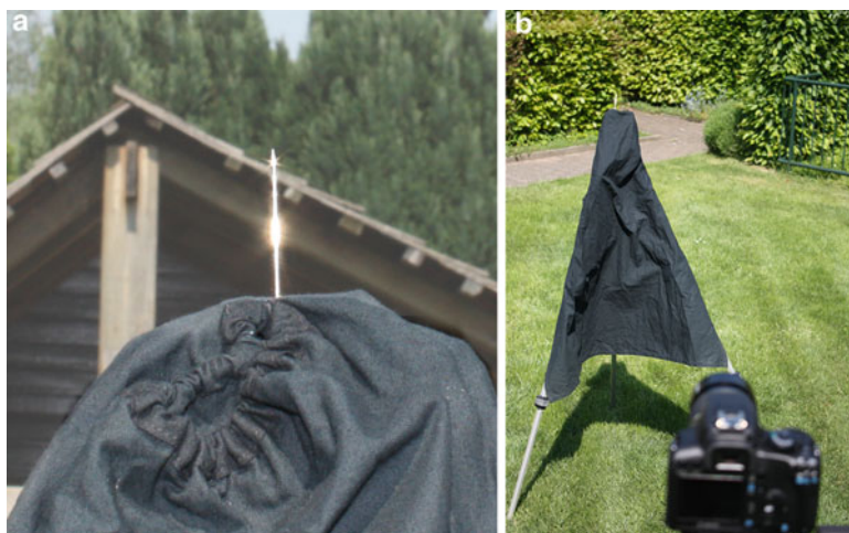
Fig. 5.3 (a) Reflective needle setup; (b) grating fitted to a DSLR and telephoto lens imaging the needle
