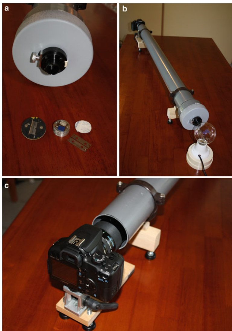
Fig. 5.1 Slit tube, showing surplus shed adjustable slit fitted. From the left: Pencil sharpener slit, disposable razorblade slit and paper slit
