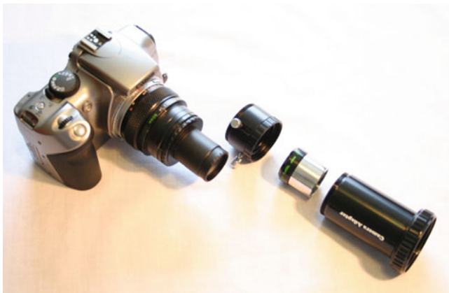
Fig. 5.11 Eyepiece projection with filter grating, showing the components
