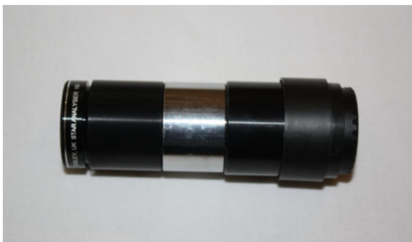
Fig. 1.6 Grating with eyepiece and cylindrical lens, ready for use
