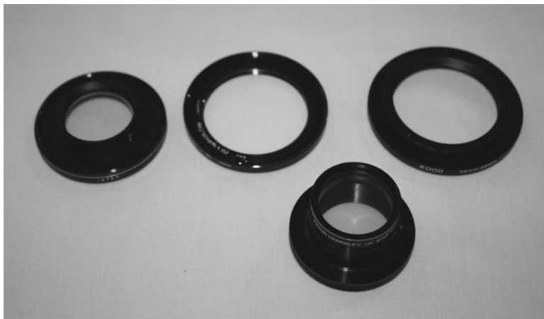
Fig. 2.13 Objective grating mounts. From the left: thin disk holding the grating in a 48 mm filter cell, T2 inner ring mounted in a 52–55 mm filter step-ring, Baader T thread to 48 mm adaptor fitted to a 48–58 mm filter step-ring. A grating mounted in a short T thread nosepiece is shown below
