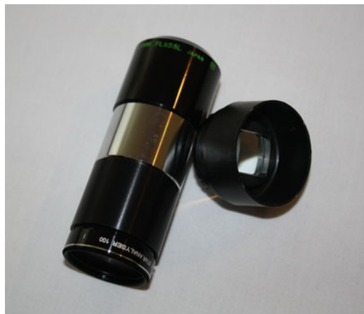
Fig. 1.5 Grating fitted to 20 mm filter extension in front of a 28 mm eyepiece. The cylindrical lens is also shown
