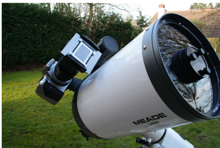
Fig. 5.16 A 35 mm objective grating mounted in a Cokin filter holder
