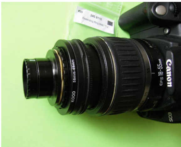
Fig. 2.9 SA100 mounted on a standard Canon zoom lens
