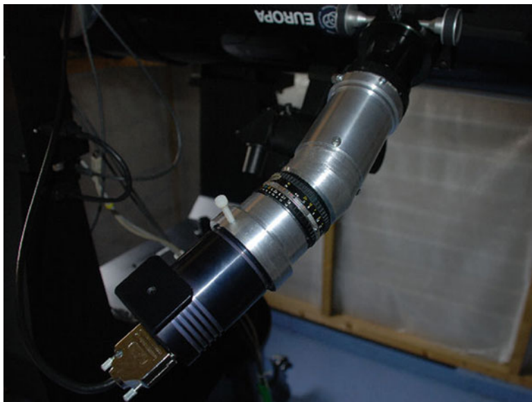
Fig. 5.20 Transmission grating spectroscope (I. Baker)
