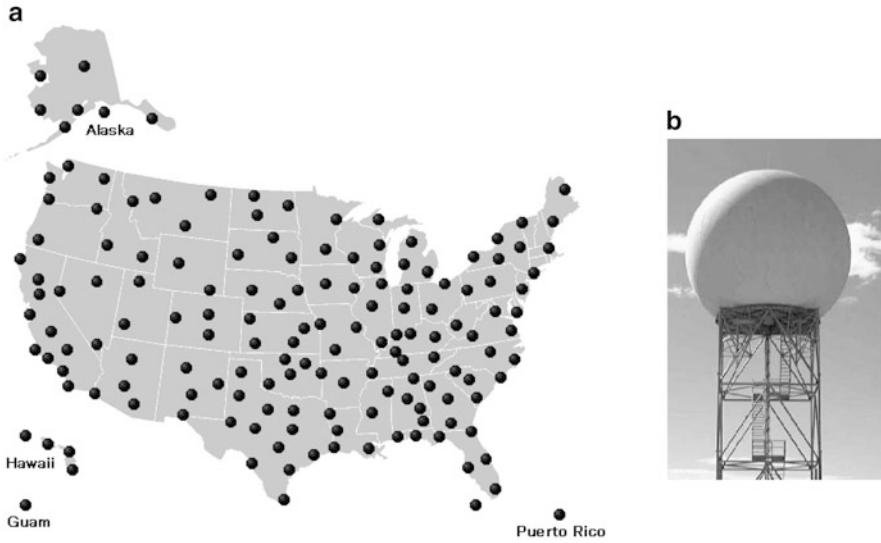
Fig. 9.1 (a) Distribution of the WSR-88D radars in the contiguous U.S., Alaska, Hawaii, Guam, and Puerto Rico [ http://radar.weather.gov/ ] and (b) the appearance of radar tower [ http://www.roc.noaa.gov/WSR88D/Engineering/NEXRADTechInfo.aspx ]
