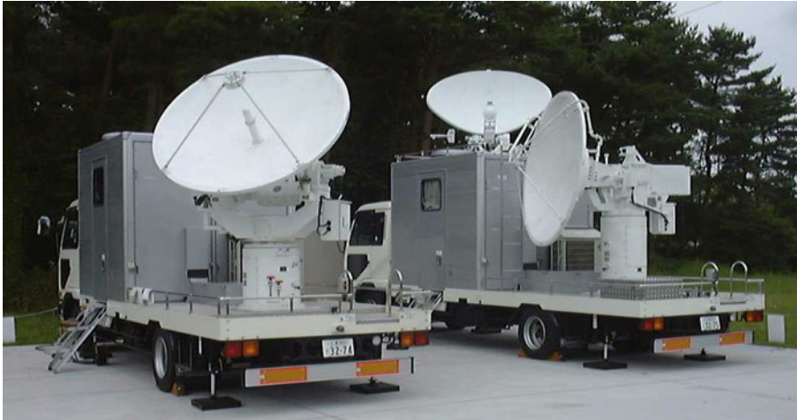
Fig. 9.9 Appearance of the 9.4-GHz radar and the satellite communication equipment for data transmission ( right-hand side ) and the 35/95 GHz radar ( left-hand side ) of NIED. The 35/95 GHz radar which will be mentioned in Sect. 9.3.2 [from Iwanami et al. 2001]
