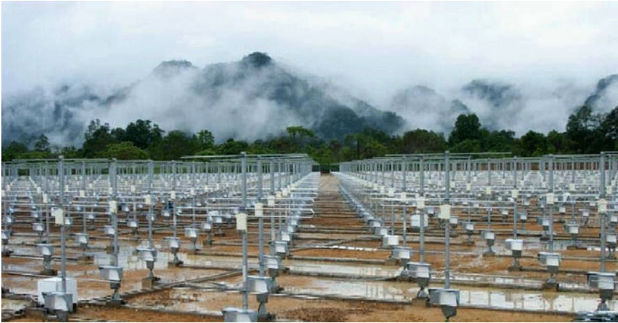
Fig. 10.9 The Equatorial Atmospheric Radar (EAR) established by Kyoto University in West Sumatra, Indonesia
