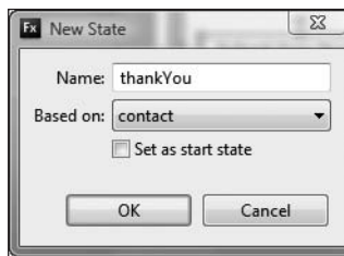
Figure 4-57. The New State dialog box for a state built over the contact state
