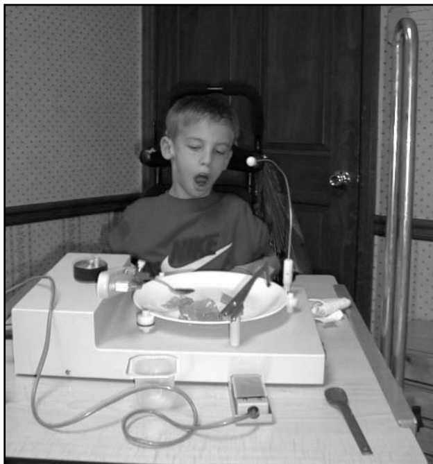
Figure 13-12. Justin can feed himself using this electronic feeder.
