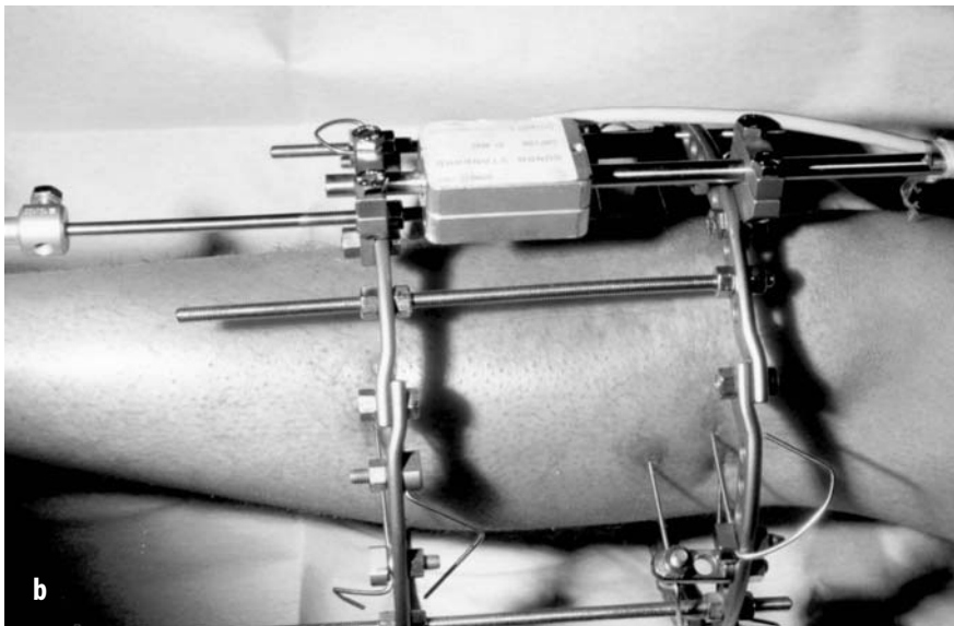
Fig. 18 a, b. Extensimetric device applied to an Ilizarov apparatus, in order to evaluate the mechanical properties of the regenerating bone
