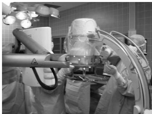
Fig. 2. Attachment of the calibration target to C-arm. A Fluoro Registration Kit is attached to the C-arm of the image intensifier
