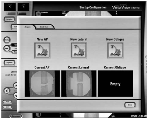
Fig. 3. Image acquisition. Fluoroscopic images in anteroposterior, lateral, and oblique views are acquired and calibrated
