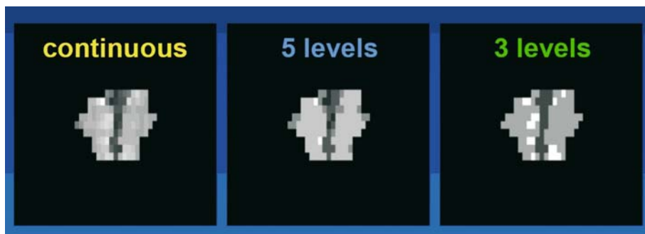
Fig. 23.2. Stratification of a continuous fluence distribution into a fluence map with a number of discrete levels
