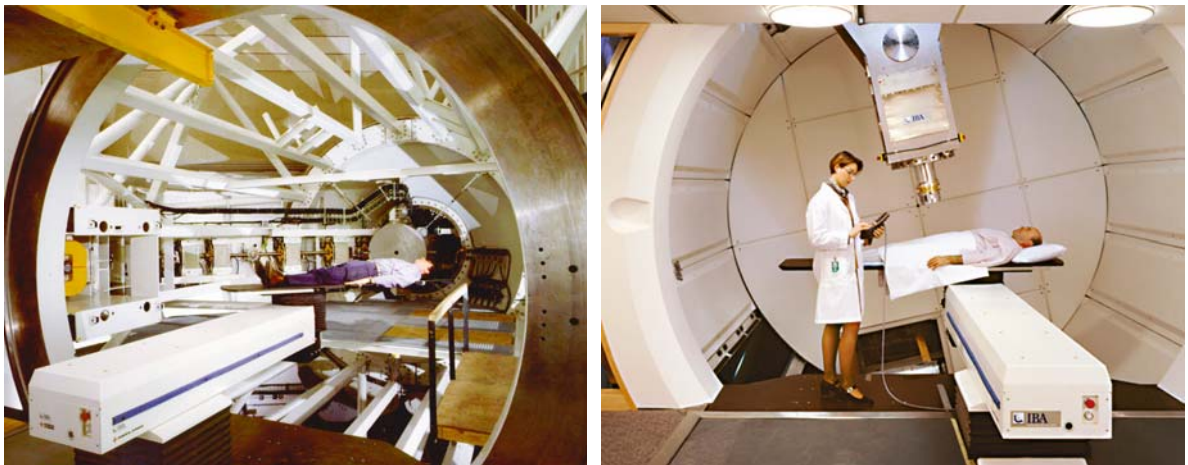
Fig. 27.7 One of the gantries at the Northeast Proton Therapy Center. Left : the gantry structure during construction with the steel assembly being visible. Right : the gantry treatment room during treatment. The beam delivery nozzle is able to rotate 360° around the movable patient couch. (Courtesy of Ion Beam Applications, S.A.).
