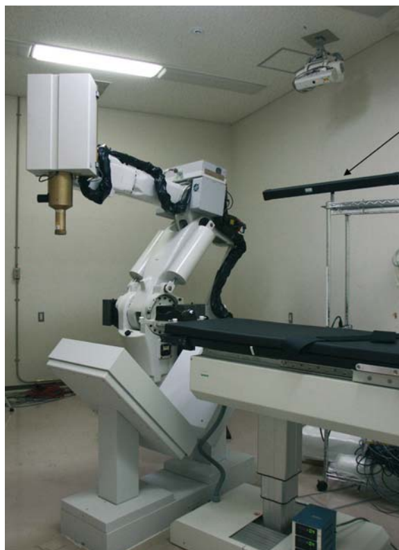
Fig. 26.2 System overview. X-ray sources, camera system, infrared tracking system (arrow)
