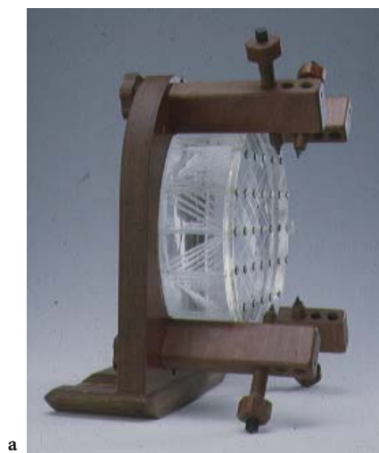
Fig. 9.2. a The three-dimensional (3D) phantom mounted in the stereotactic guidance system for measuring 3D position of MR imaging plane. This is comprised of a regular grid of water-filled rectangular boreholes, with oblique water-filled boreholes in between. This produces a pattern of reference points surrounded by measurement points in axial image from which the 3D position of the imaging plane can be reconstructed. b A 3D-phantom measurement. The distance d between reference point (rectangular water-filled borehole) and measurement point (oblique water-filled borehole) is a direct measure of the z coordinate of the imaging plane at the reference point, since the angle between oblique water-filled borehole is \alpha=2 \arctan (0.5) . Systematic discrepancy in the distance measurements of d_1>d_2>d_3>d_4>d_5>d_6 would be detected if the imaging plane were tilted. c Axial image of the 3D phantom. The 3D position of the imaging plane can be reconstructed from the measured points. d Typical example of the 3D position of the imaging plane with properly adjusted shims. Deviations in z direction are reduced to about 1 mm which approximates again the dimensions of the image pixels (1 mm slice thickness). Mathematical correction of these discrepancies in the z direction was not pursued since properly adjusted shims avoid deformation or tilting of the imaging plane. e A tilting of the 3D phantom of about 3^\circ from transversal to sagittal and coronal direction can be clearly detected. (From SCHAD 1995)
