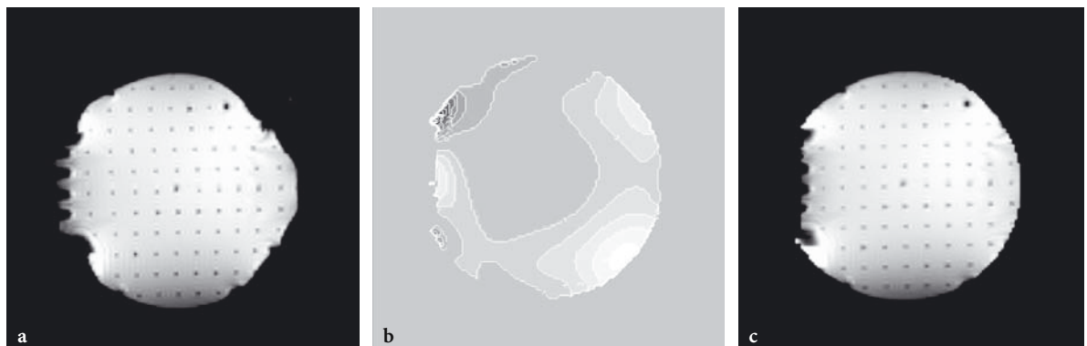
Fig. 9.3a–c. Correction of local MR image distortion using echo-planar imaging (EPI) measurements. a Original EPI phantom image of a water-filled Plexiglas cylinder with a rectangular grid of plastic rods. b Corresponding field map. c Field-map-corrected EPI image. (From SCHAD 2001)
