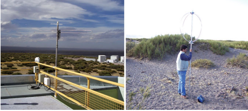
Fig. 5.1 Left preliminary test beacon at the roof of Coihueco; right measurement of the beacon power at the AERA site with a mobile, 1 m diameter SALLA on a 3 m pole and a spectrum analyzer
