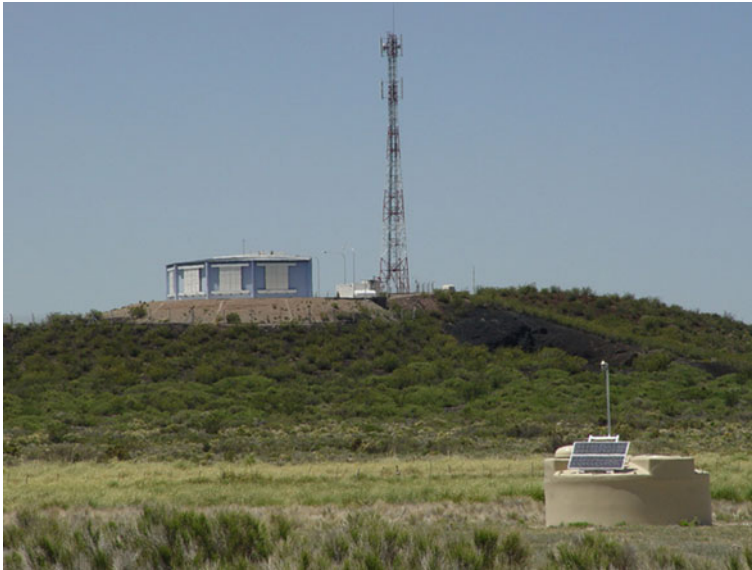
Fig. 3.6 Fluorescence telescope building and water Cherenkov detector of the Pierre Auger Observatory in Argentina Published with kind permission of © the Pierre Auger Collaboration 2010 ( http://www.auger.org/media/ )
