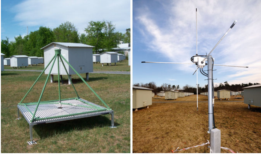
Fig. 3.2 Left Inverted V-shaped dipole antenna type used in the LOPES 30 east-west and dual polarized setups. Right Tripole antenna type used for the LOPES 3D setup. Published with kind permission of © the LOPES Collaboration 2005, 2010 (published, e.g., in Refs. [63], respectively [30]).
