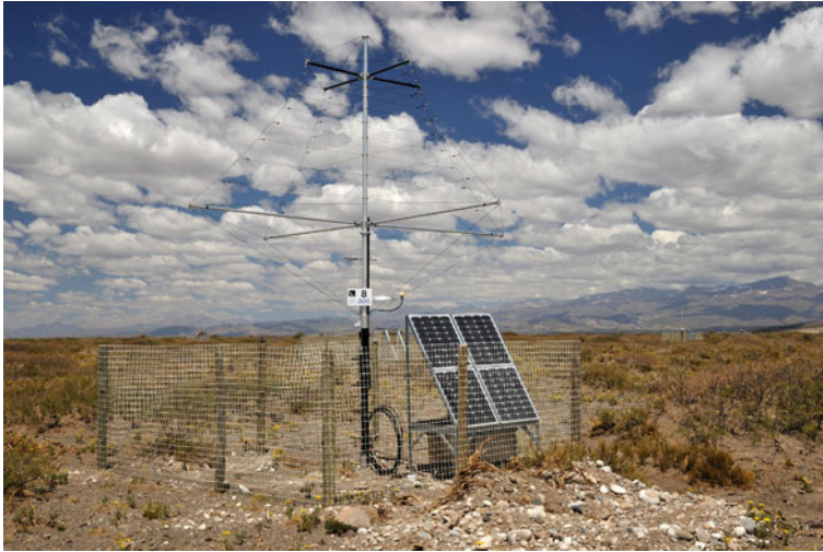
Fig. 3.8 AERA station with wired LPDA. Published with kind permission of © the Pierre Auger Collaboration 2010
