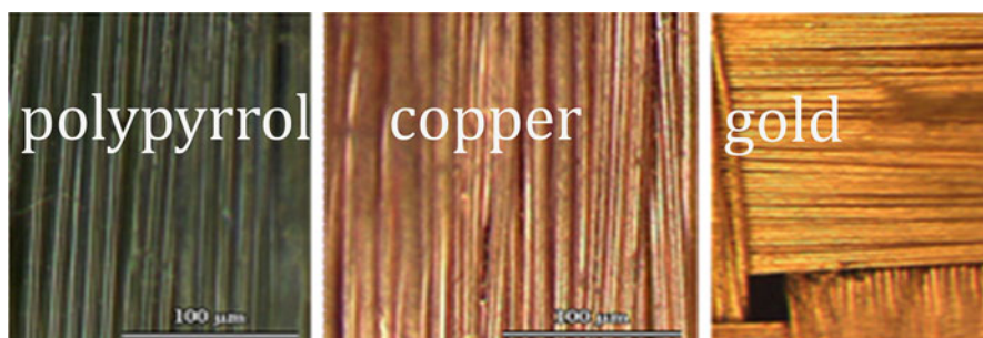
Fig. 6.1 Kevlar fibres coated with conductive materials
