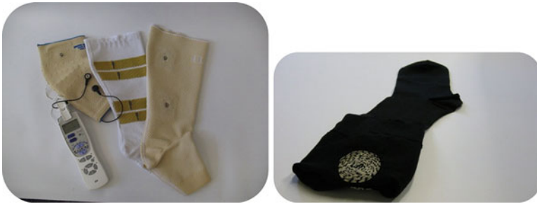
Fig. 6.6 Textile products with embedded actuators
