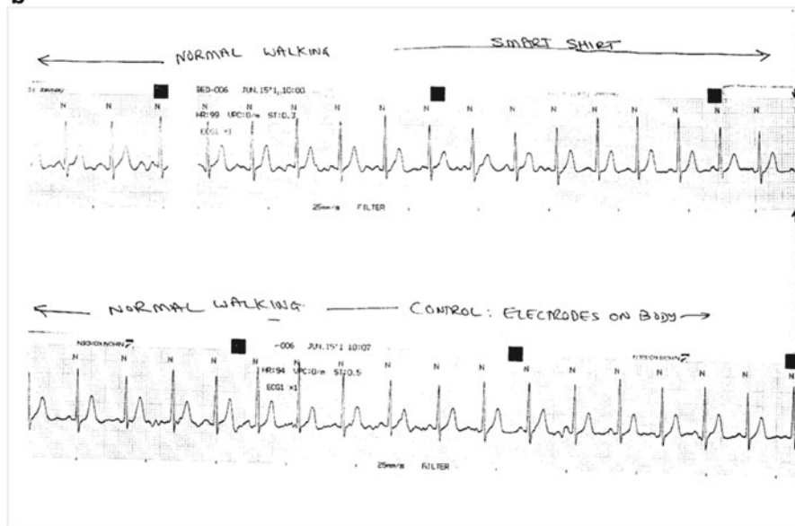
Wireless Transmission of Vital Signs Top Trace: From the Smart Shirt Bottom Trace: Directly from the User
