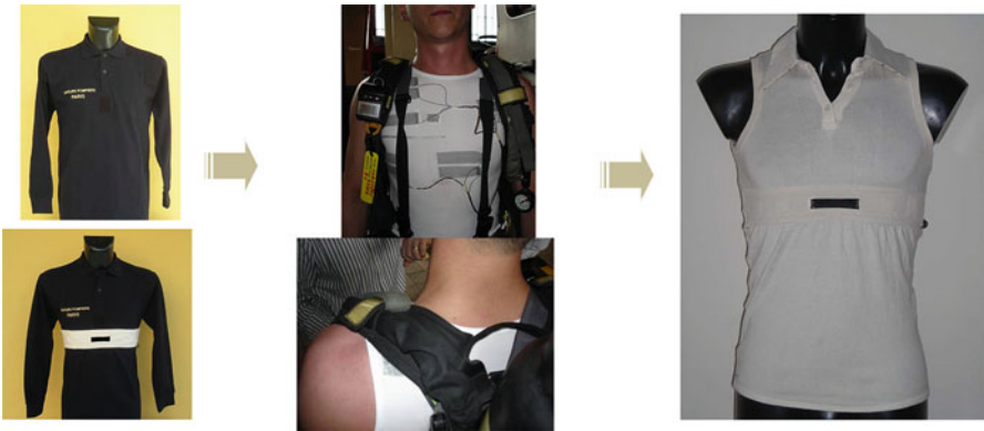
Fig. 6.15 The evolution of the Proetex inner garment
