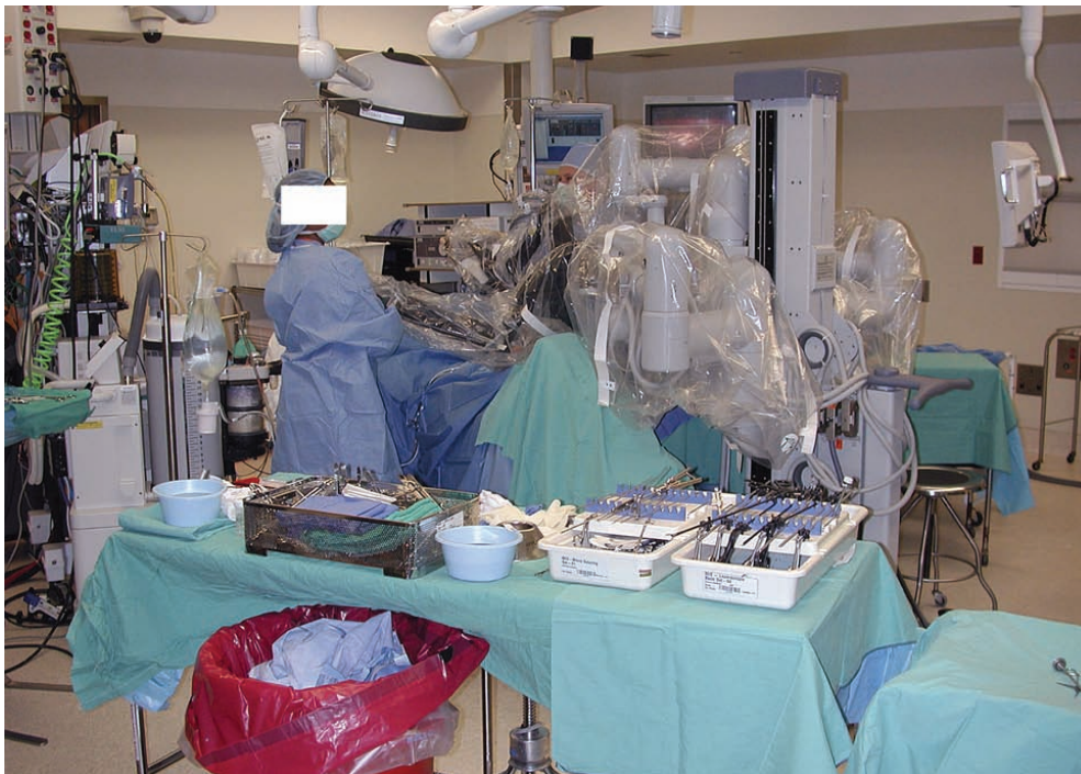
Figure 38.5 Typical operating room set-up of the robot. The tower is placed between the patient's legs and the robotic arms are attached to the instruments in the lateral ports
