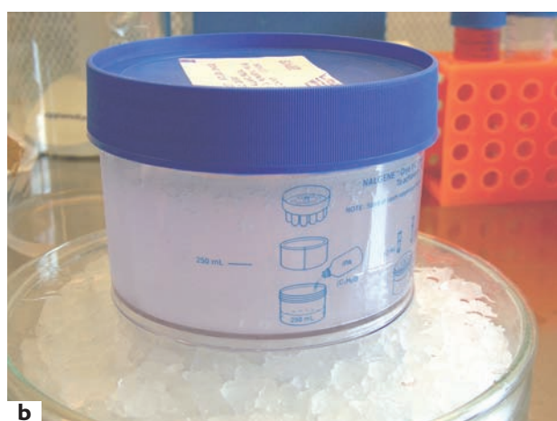
Figure 29.3 (a) Ovarian perfusion through the ovarian artery. (b) Passive cooling device (5100 Cryo 1°C freezing container)
