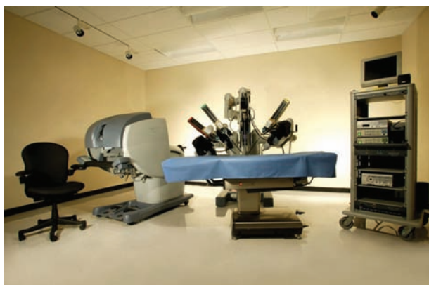
Figure 38.1 The complete robotic unit consists of a console, the robotic tower and the video cart. Courtesy of Intuitive Surgical
