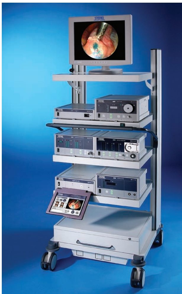
Figure 2.21 EndoCart™ set-up, including: flat screen monitor, digital camera, xenon light source, insufflator, suction-irrigation system, Aida DVD recorder (for digital storage of still images, video sequences and audio files) and motor system for morcellator
