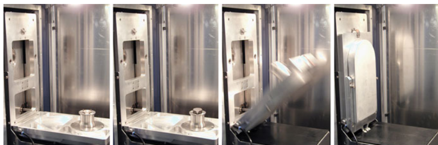
Fig. 17.8 Operation of sample stand shown in a sequence of four steps. From left to right: (a) The pivoting plate is in horizontal position ready to take over the production control sample. (b) The sample is put onto the sample support. (c) The pivoting plate moves into an upright position. (d) The pivot plate has reached the vertical position and is in contact with the connecting plate. The sample is fixed onto the rotating disk and the measurement starts
