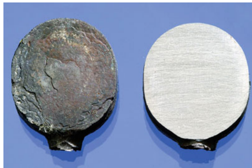
Fig. 17.1 Production control sample, left : original appearance with scale layer, right : after grinding; width of the sample: about 35 mm
