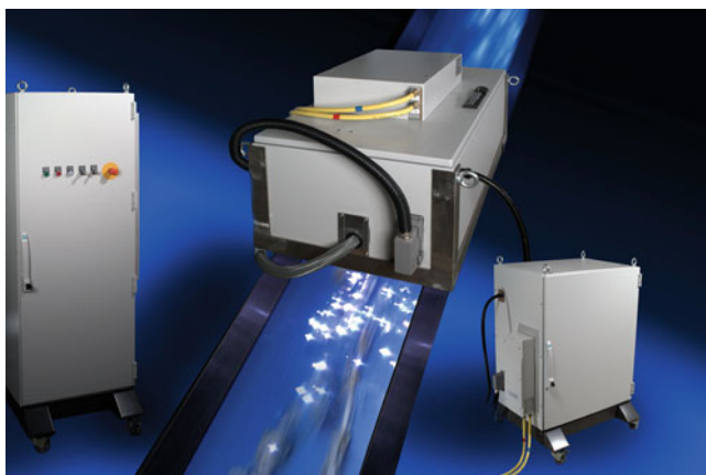
Fig. 18.24 System for the identification of scrap pieces on belt conveyors. Left: electric control cabinet, middle: laser module mounted above the belt conveyor with scrap pieces and laser-induced plasmas (time exposure showing a multitude of laser-induced plasmas), right: spectrometer module
