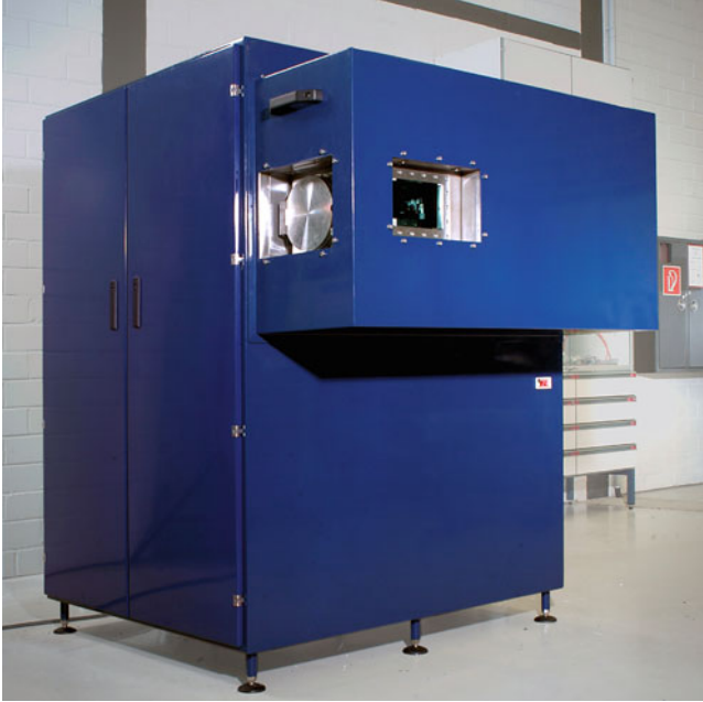
Fig. 18.10 High-speed scanning LIBS microanalysis system SML to measure steel samples for the analysis of segregations, inclusions, and decarburization zones
