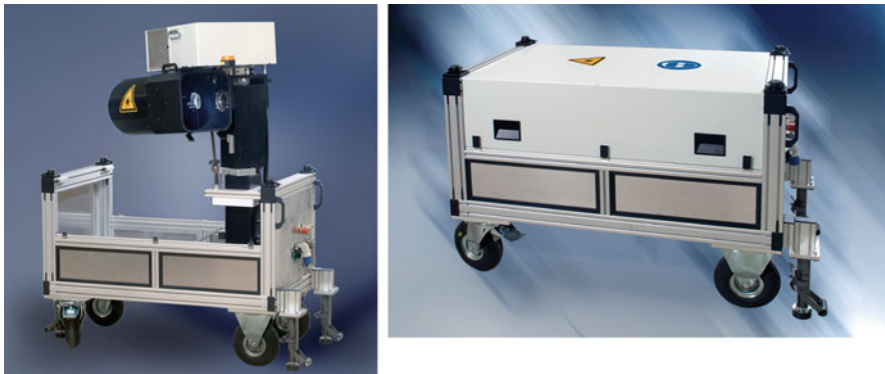
Fig. 17.27 Left: Remote LIBS system TeleLis with the optics in the position ready for measurement. Right: TeleLis system ready for transport
