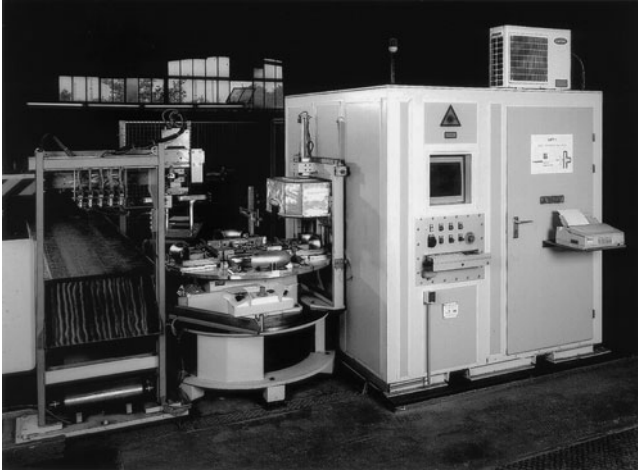
Fig. 17.14 First LIFT inspection system installed in the production plant. Right: inspection system, middle: table type circular conveyor to feed the pipe fittings, left: belt conveyor to transport the inspected parts to the packaging line, cf. Fig. 17.13
