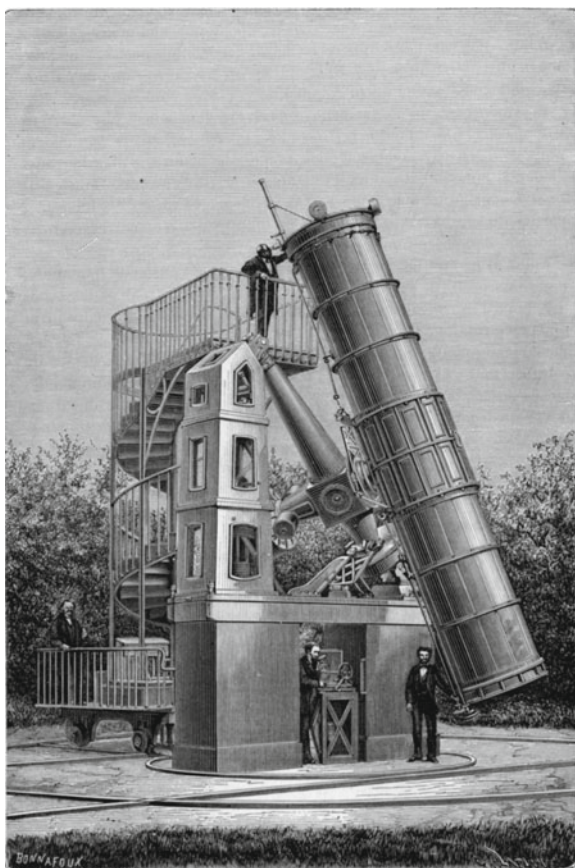
Fig. 7.11 The telescope of 120 cm diameter at the Paris Observatory. The mounting is of the Newtonian type, the observer places himself at the side of the upper end of the tube, the light is concentrated by the main mirror and deflected by a small flat mirror set at a 45 degree angle into the eyepiece. The observer uses a mobile staircase that can be adjusted to different heights. When not in use, the telescope is protected by means of a rolling shelter
