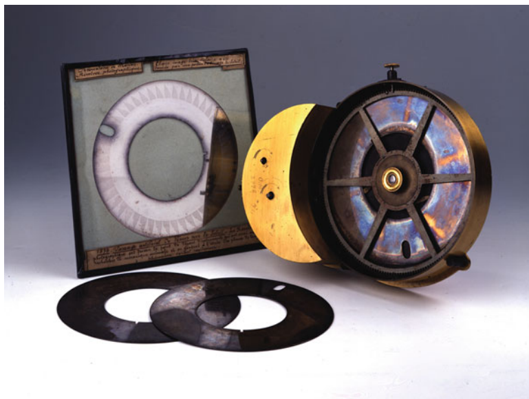
Fig. 5.26 Janssen's "revolver photographique" (For a detailed description, see Flammarion C. Le passage de Vénus, résultats des expéditions françaises , La Nature , 1 er semestre, pp. 356–358 (1875)). This apparatus contains a circular glass photographic plate that can advance in jerks in order to take successive images of the same object at regular intervals. It was used by Janssen in 1874 to observe the passage of Venus in front of the Sun. This is one of the ancestors of the Lumière brothers' cinematograph (and Janssen himself was one of the first subjects)
