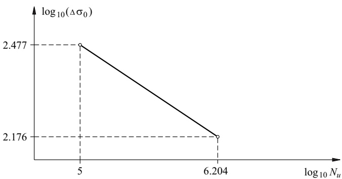
Fig. 7.17 S-N curve for example 7.5
