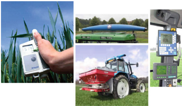
Fig. 12 N-tester and N-sensor: Time- and crop-specific nitrogen fertilization. From Yara/Agricom
