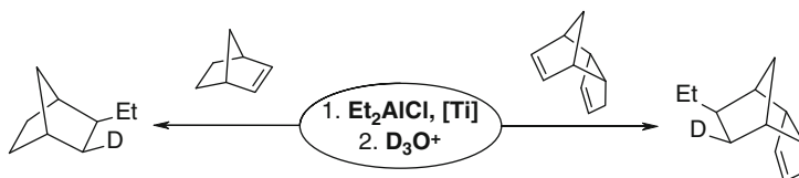
Scheme 11 Ti-Catalyzed hydroalumination of norbornenes by \text{Et}_2\text{AlCl}
