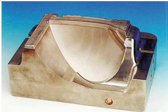
Fig. 5.13 Modification of an injection mold for a car lamp housing (material: hot working steel) [5]
