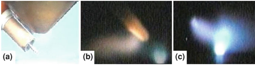
Fig. 10.33 Images of a laser nozzle/electrode assembly, b arc, deflection away from laser-generated plasma due to co-axial gas jet and c arc-plasma coupling with Argon cross-jet
