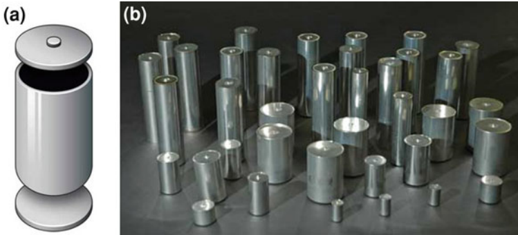
Fig. 4.50 Laser welding of lithium ion batteries, a Schematic of various components to be welded, and b welded batteries of different sizes [66]
