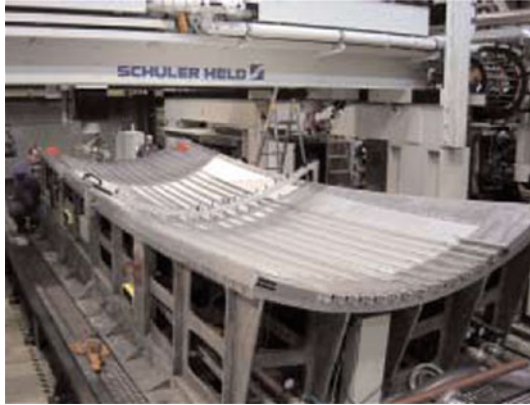
Fig. 4.51 Fixture for laser welding of stiffeners to fuselage skin [67]
