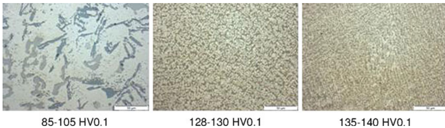
Fig. 5.3 Grain refinement in the alloy AlSi10Mg after laser remelting [16], P = 1\text{ kW} , d_L = 1\text{ mm} ; left substrate, centre v_v = 0.5\text{ m/min} , right v_v = 5\text{ m/min}
