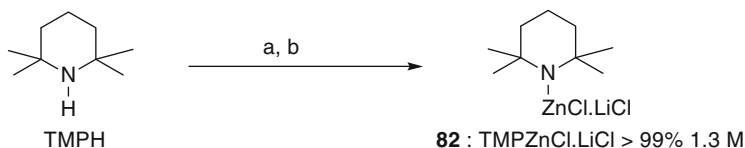
Scheme 29 (a) 1.1 equiv n -BuLi, THF, -40^\circ\text{C} to -10^\circ\text{C} , 1 h, (b) 1.1 equiv \text{ZnCl}_2 , THF, -10^\circ\text{C} , 30 min then 25^\circ\text{C} , 30 min [74]
