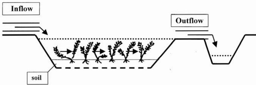
Figure 4-14. Schematic representation of a constructed wetland with submerged macrophytes. From Vymazal (2001a) with permission from Backhuys Publishers.
