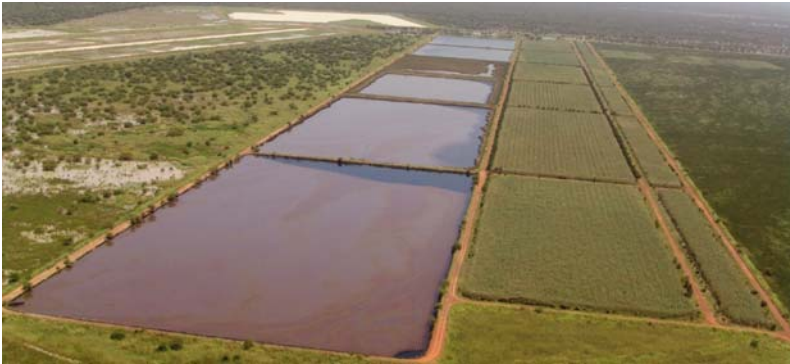
Figure 6-1. HF constructed wetland at Heglig, Sudan planted with Phragmites australis treating hydrocarbon contaminated water from the oil fields. Photo provided by Oceans-ESU Limited, United Kingdom, with permission.
