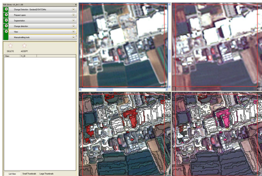
Fig. 6.4 An example of change detection processing performed on eCognition platform. Top: images acquired at dates T0 and T1. Bottom left: change detected automatically, bottom right: change accepted manually. Automatically detected changes ( red patches in the bottom left panel ) are assessed by the operator as real (new building in the middle ) or seasonal (agricultural parcels in the left ). Only the first one is accepted in the final change/no change map ( bottom right )
