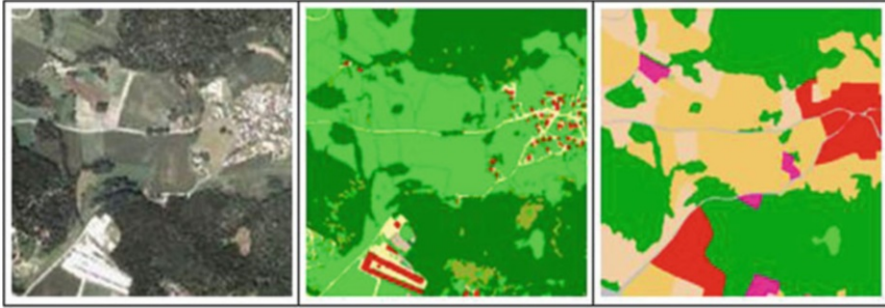
Fig. 15.2 Land use map (surrounding of City of Klagenfurt, Austria) ( left : orthophoto 2009, middle : land cover map, right : land use map)
