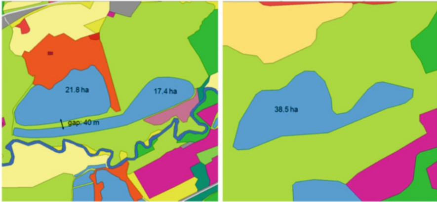
Fig. 16.6 Gap between two lakes (DLM-DE/CLC 1 ha – left side , © BKG/Geobasis-DE) that has to be closed during generalization in comparison with CLC2006 ( right side , © EEA 2006)
