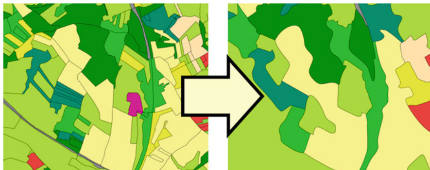
Fig. 16.7 Results of generalization from 1 to 5 ha (DLM-DE2012 – left side 1 ha, right side 5 ha , © BKG/Geobasis-DE)
