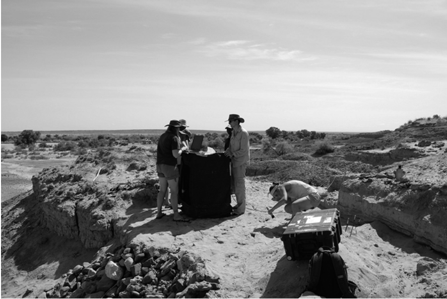
Fig. 2.10 Optical laser scanner in the field protected by a canvas cover around a square frame made of carbon fibre as shown in Fig. 2.9b. The image shows the authors scanning human tracks at Ileret in 2009
